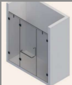
ONE DOOR AND TWO FIXED PANELS (STRAIGHT)
